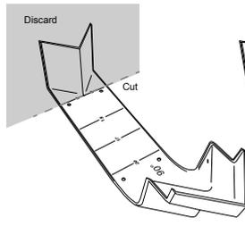
Option to extend Cast Angles to fit Quad Gutter 150, 175, or 200mm (175 illustrated)
